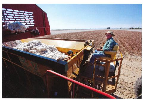
Andrews operates the module builder, which compresses the cotton for pickup. During picking, cotton is transported to the builder by boll buggies, allowing the two pickers to operate continuously in the field.
