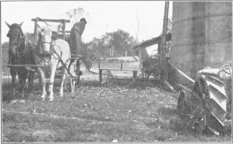
Fig. 13.—The small farm tractor has plenty of power to cut and elevate silage much faster than is usually necessary or desirable on the average farm, provided a good cutter is used and it is properly adjusted and is run at the correct speed.
