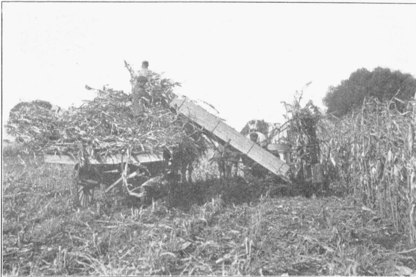
Fig. 5. A bundle elevator on the binder will eliminate much hard work, although it may not reduce the cost of silo filling.
