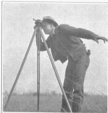
A young farmer in Cooper county learning to use the farm level at a county extension school for soil conservation leaders.
