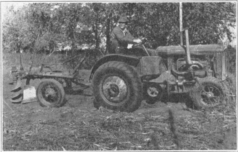
Fig. 13.—The Whirlwind Terracer. Picture by courtesy of the Soil Conservation Service.
