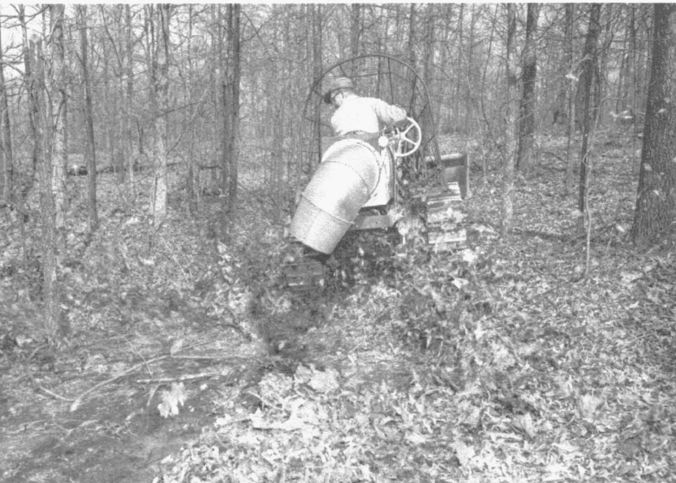
Blower crossing area shown in picture above at a speed of 0.75 mph. Air blast cleans leaves from around sprouts. Debris in motion indicates power of air blast.
