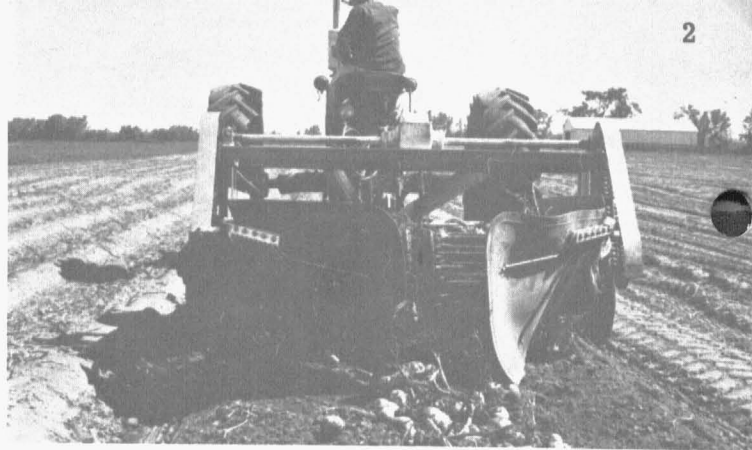
This series pictures steps in a typical commercial harvesting operation. (1) Vines are destroyed a few hours before harvest with a mechanical vine beater. (2) Two-row digger windrowing tubers into a single
