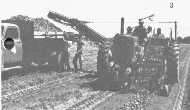
row. (3) Potatoes are then elevated and bulk loaded for transport to grading shed. (4) Vines, clods, and other debris are removed in the field by a crew riding on the elevator.
