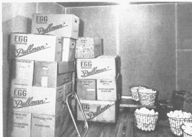
Fig. 3—Cool room (45° F. to 50° F.) made from a used Smith incubator. Capacity is 200 thirty-dozen cases. Note dolly used for stacking and moving eggs.
