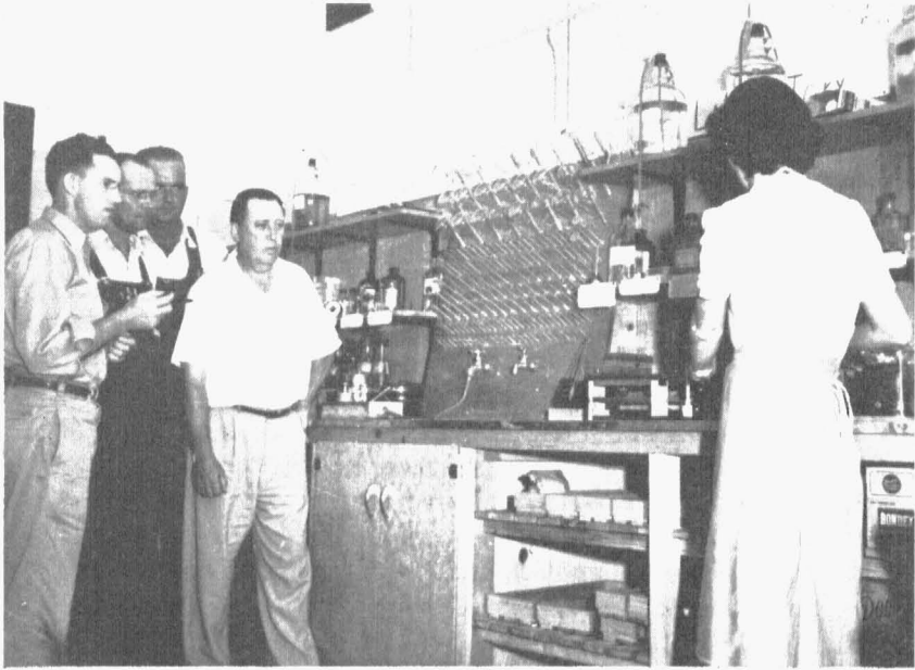
Fig. 3. One of Missouri's 85 county soil testing laboratories, showing the county agent and laboratory technician making and interpreting the tests of soil samples submitted by local farmers. This service enables each farm operator to balance his fertilizer applications to fit the needs of each crop and each field.
