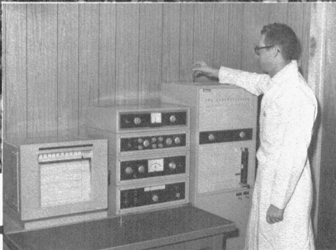
◀ Graduate student Kenneth Read collects soil cores in path of implement and tests extract from them (inset) in gas chromatograph for fertilizer placement.
