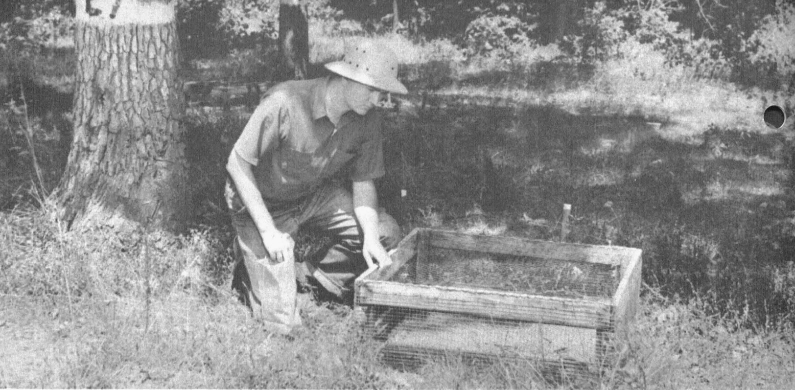
An acorn trap is pictured in position under the crown of a white oak. The trap is 3.3 feet square. It is covered with chicken wire and has hardware-cloth bottom and sides.
