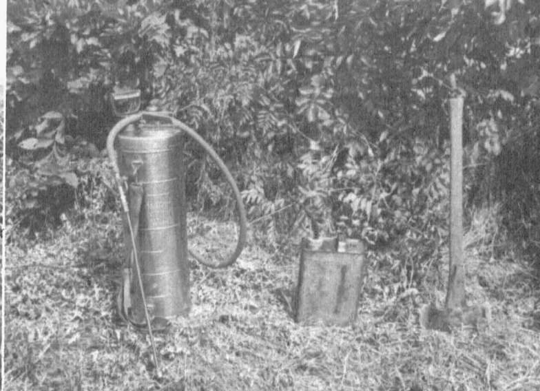
Figure 4—Sprayer, pouring can and axe: the brush killer's tool kit. Disposable cans are best for ammate as it rusts sprayer parts.
