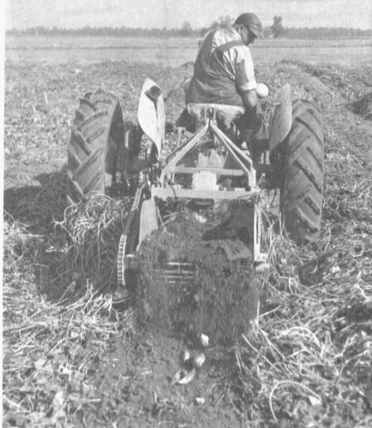
Fig. 5—New, improved models of sweet potato diggers and lifters are overcoming the problem of bruising that made early models unsuccessful.
