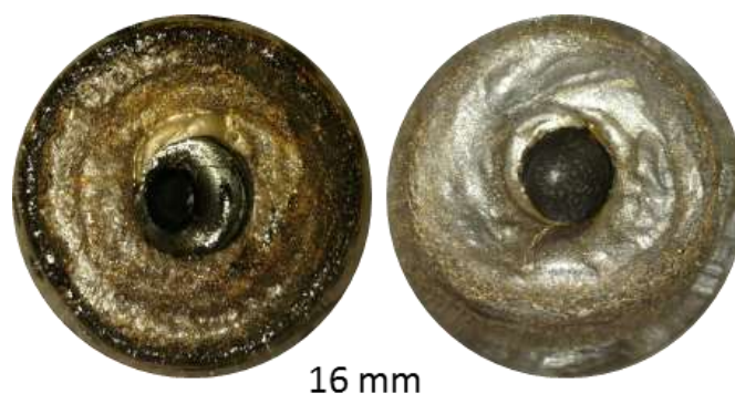
Figure 8. Lobate surface structures observed in quenched concentric cylinder run products may suggest yield strength development. These surface structures are only observed at the lower temperature experiments. Examples are given above for structures found in both Nyiragongo (right, 1145^{\circ}\text{C} ) and Nyamuragira (left, 1165^{\circ}\text{C} ) compositions.
