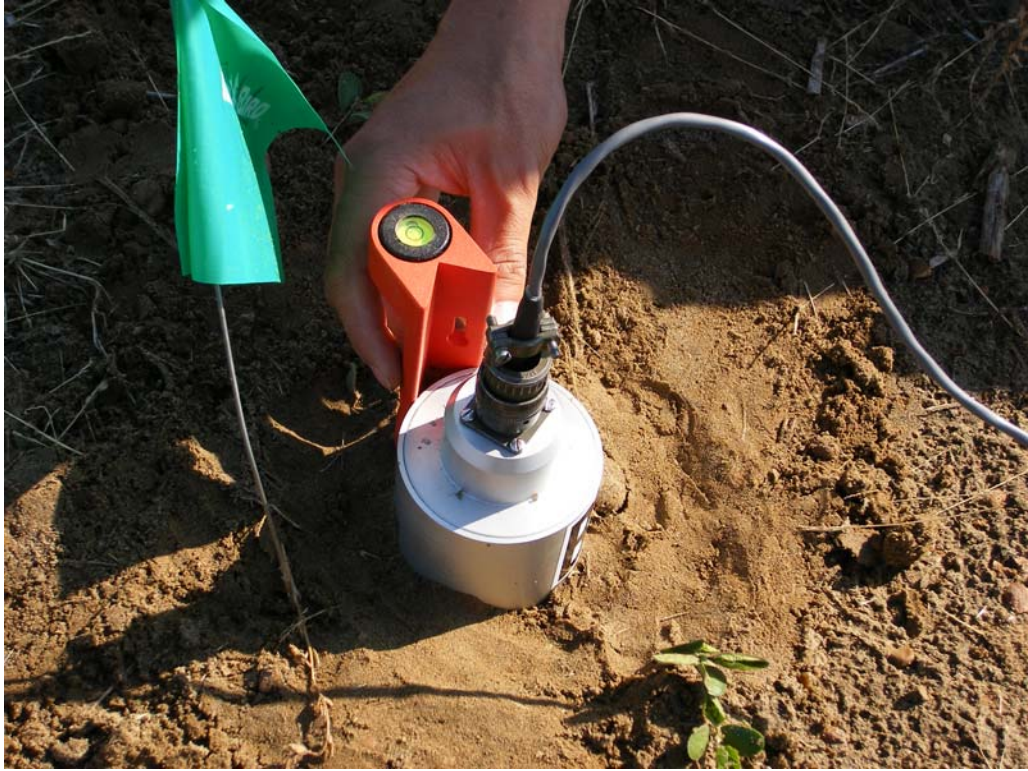
Figure 4. 6 Photograph of 1-Hz geophone Placed in the Ground and Leveled.
