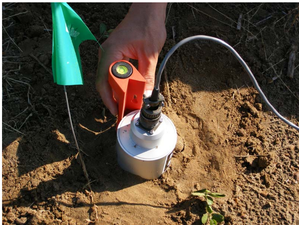
Figure 5.4 Photographs of Geophone and Surficial Soil at Site 1.
