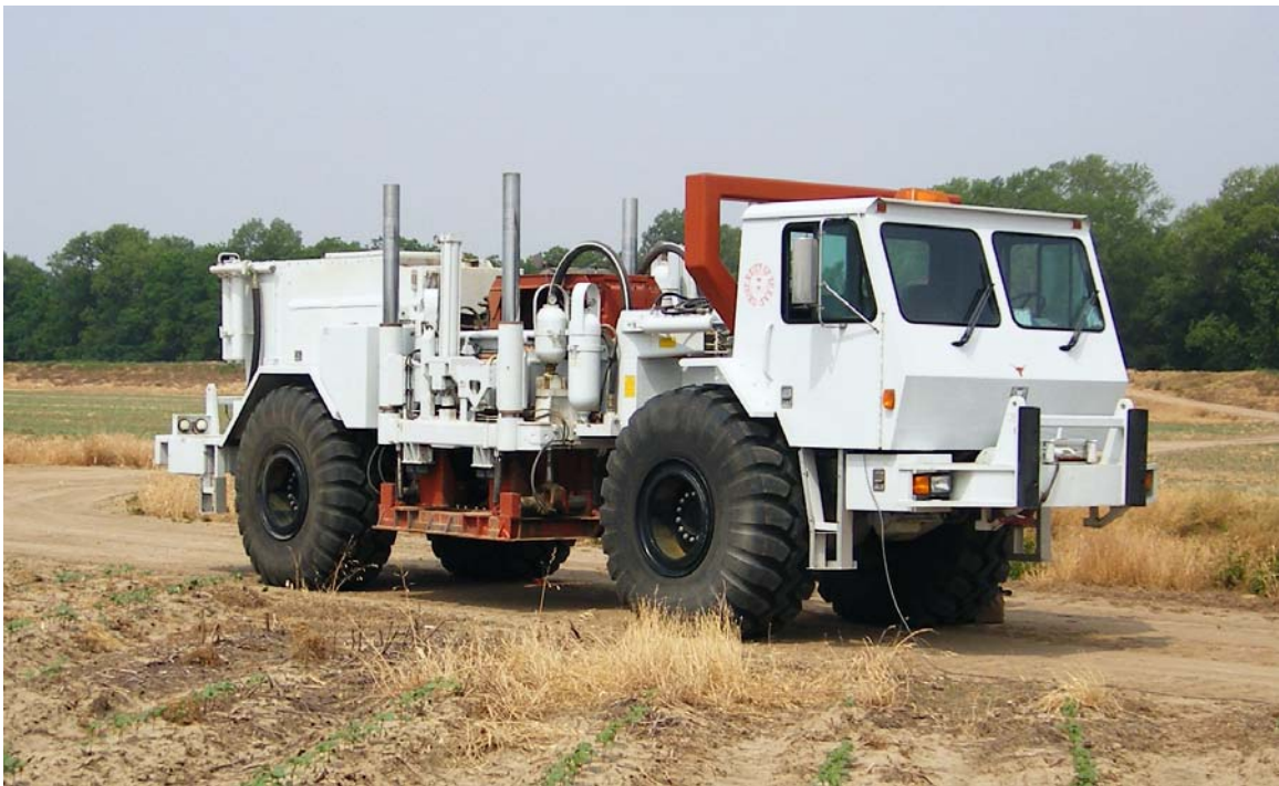
Figure 4.4 Photograph of Low Frequency Mobile Shaker “Liquidator” developed as part of the Network for Earthquake Engineering Simulation (NEES) Program.
