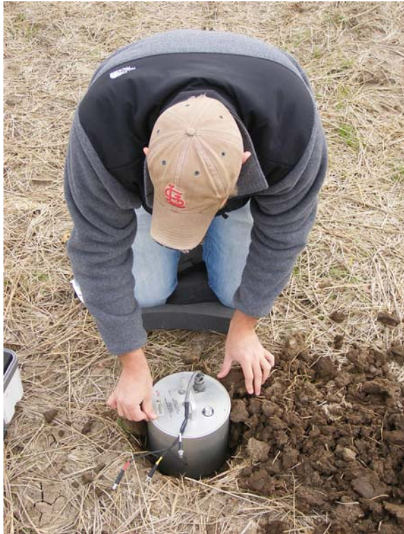
Figure 4. 15 Photograph of the 3-Component Geophone Being Placed at Site 5.
