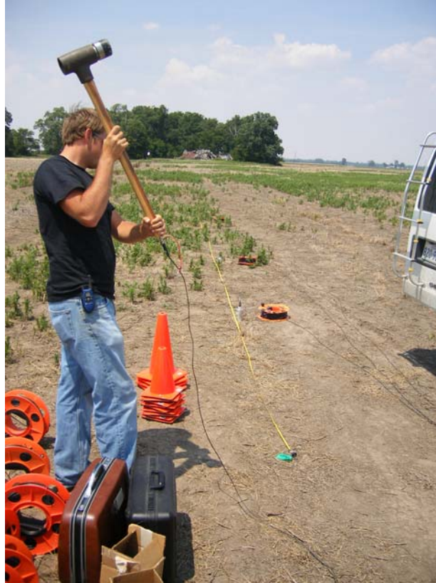
Figure 4.3 Photograph of Instrumented Sledgehammer Used to Excite High Frequency Energy.
