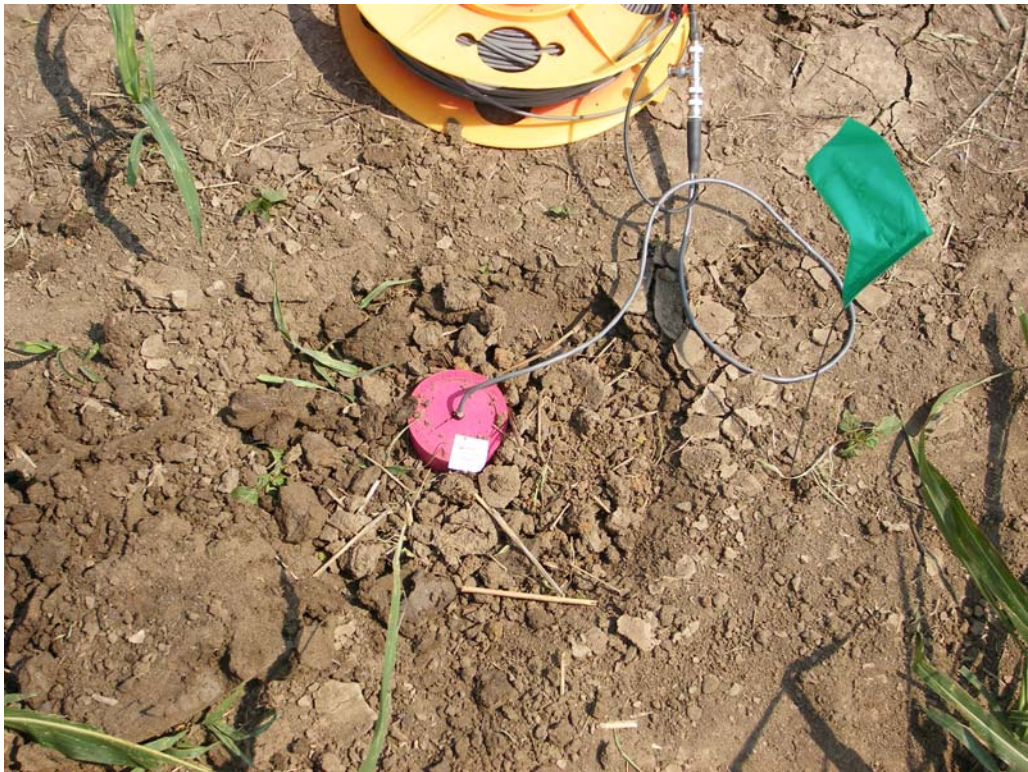
Figure 4. 7 Photograph of 1-Hz Geophone Buried and Insulated to Maintain Low Operating Temperature.
