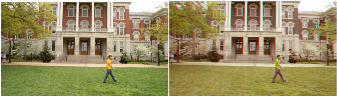
Figure 7.7: Creating stereo video from 2D-3D Registration. Left: Original video frame. Right: After video is registered with range scan, the 3D location of video pixels are known. Images for the left and right eyes can be created and combined to create an anaglyph image. (Best viewed with 3D anaglyph glasses.)
