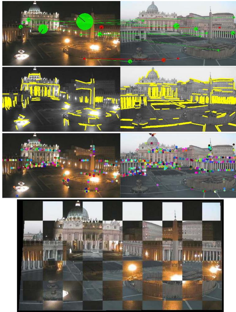
Figure 3.9: Using Pseudo Corners to align a difficult image pair, called Vatican. Top: The majority of the SIFT (green) and linearly-verified (red) keypoint matches for this pair are incorrect and cannot be used to align the images. No SIFT+HOG matches were identified in this example. The relative SIFT scales are represented by the size of the circles and the features' orientations are denoted by the black lines. 2nd Row: Line segments extracted from images (shown in yellow) that are used to find Pseudo Corners. 3rd Row: Pseudo Corners identified after intersecting line segments. Bottom: Image pair is aligned using the homography calculated from the matched Pseudo Corners.
