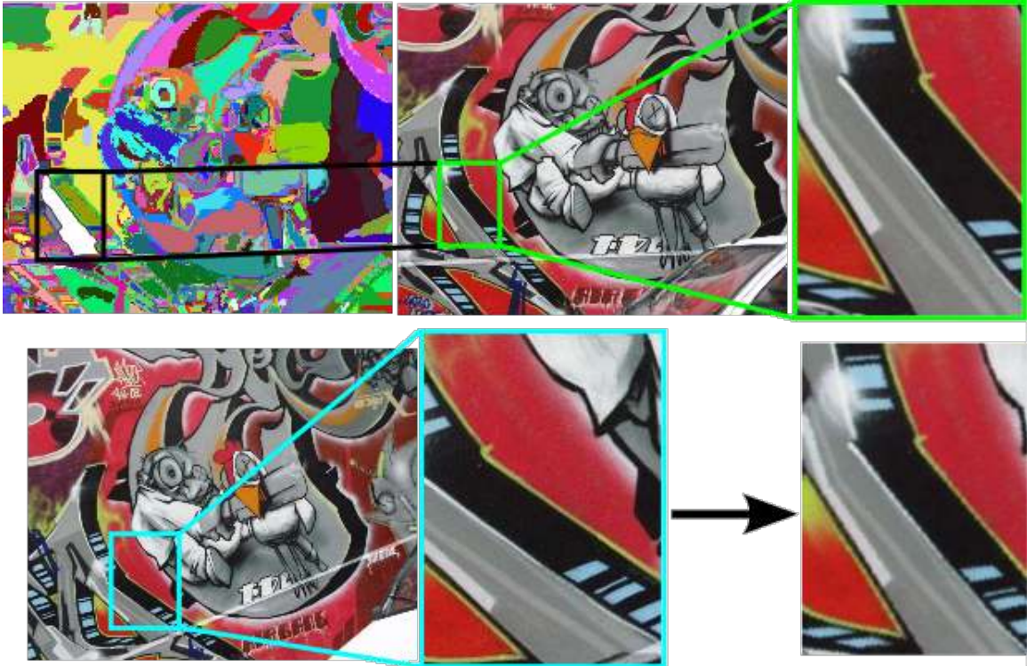
Figure 3.4: Mapping bounding box of MSER neighborhood in I_1 to I_2 . Top : MSER segments and MSER defined neighborhood in I_1 . MSER segment being used is shown in white. Bottom : Original MSER neighborhood in I_2 and I_2 's patch after it has been transformed to the same coordinate system as I_1 's patch via a scaling and rotation. The patch in I_2 is extracted at multiple scales and each patch is rotated such that its x-axis points along the dominant gradient direction in the patch.
