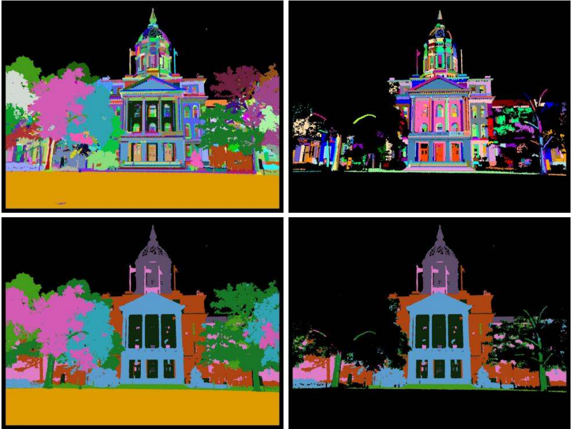
Figure 5.1: 3D segmentation images. Top left: Initial 3D segmentation results. Top right: Initial segmentation with segments marked as ground or trees removed. Bottom left: Initial 3D segments merged into ten main clusters. Segments are merged based on 3D depth. Bottom right: Main clusters after those that have voted themselves to be ground or trees are removed.
