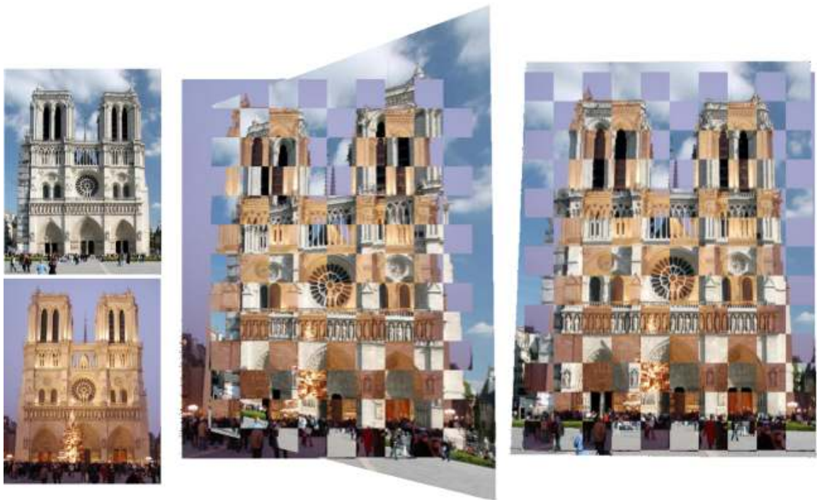
Figure 3.8: Image alignment improvement using our ensemble SIFT method. Left: Image pair to be aligned. Center: Image alignment using only SIFT features. Right: Image alignment using our ensemble features.
