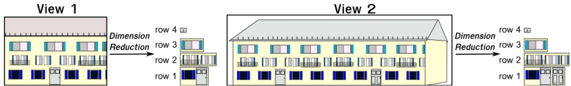
Figure 4.3: Overview of how we use dimension reduction to represent an image. Repetitive and salient regions are searched for along the horizontal axis and a single representative patch for each group is chosen. By first focusing on just aligning the representative patches extracted from different images in just one dimension, we remove the ambiguity caused by attempting to match repeated elements across images.
