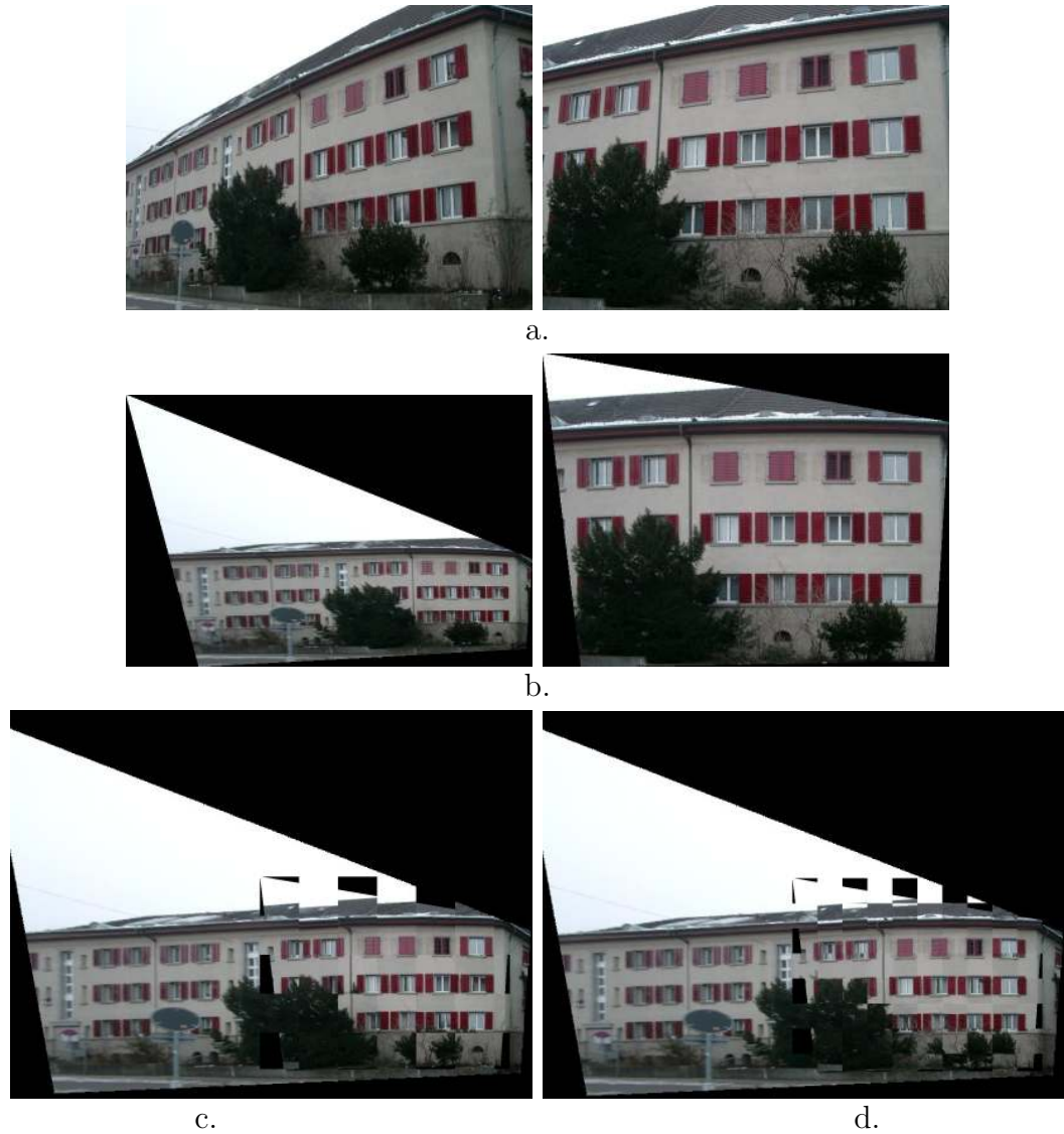
Figure C.9: Example of radial distortion-induced errors. a) The images in this pair from the ZuBuD dataset (object0111:view01-view03) exhibit radial distortion which prevents from them being b) accurately rectified. With this type of warping, even the c) ground truth homography which is shown here is not 100% correct. This leads to some inaccuracies in our evaluation because the ground truth and all of the methods tested on radially distorted images suffer from homography errors due to this warping in addition to any keypoint or region match inaccuracies. d) We show the aligned result of our full pipeline to visually compare with the ground truth result.
