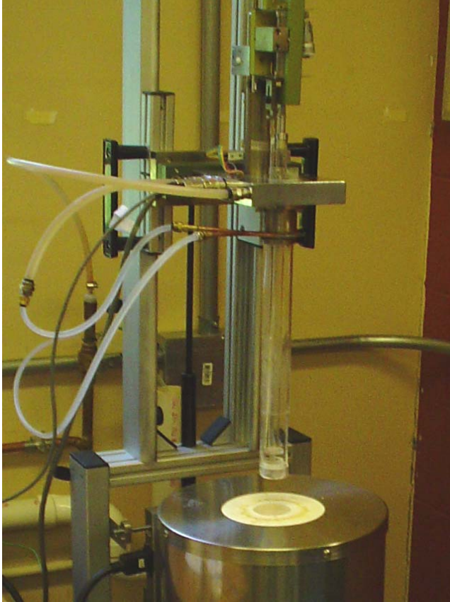
Figure 3.1. The parallel plate viscometer setup (left). A \eta - T datum is gathered by placing a cylindrical core (below) under a known stress, and measuring its linear deformation rate at a stable temperature.
