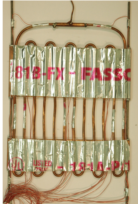
(b) Photo of an OHP with thermocouples attached.
