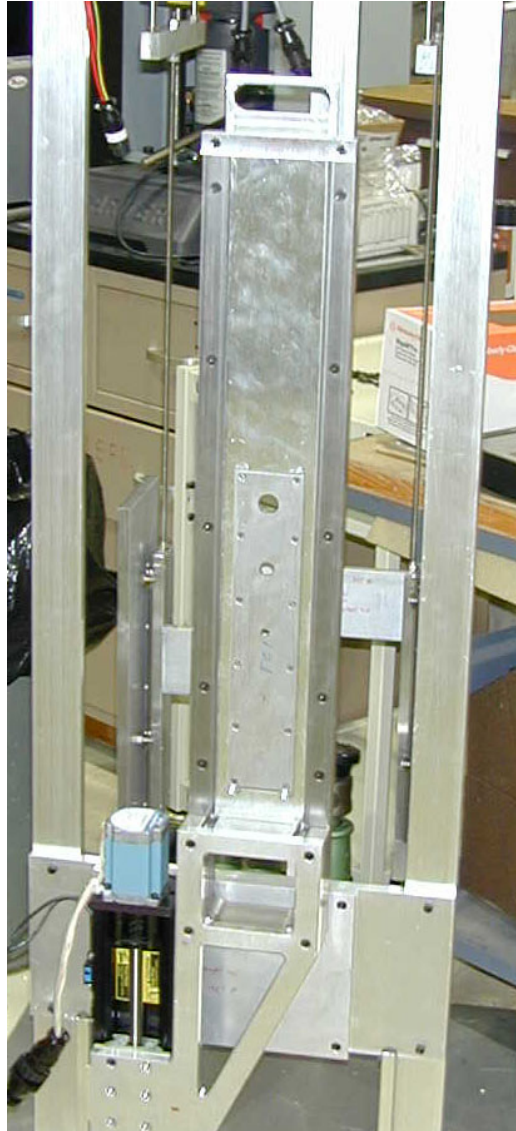
Figure 3.5. Aperture assembly for the Neutron Imaging beam line (Jacobson 2007).
