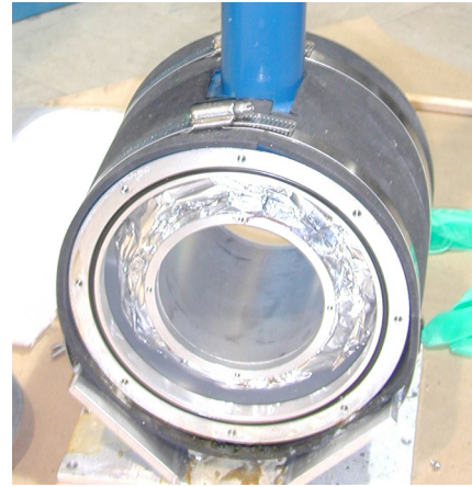
Figure 3.4. Dewar used on the Neutron Imaging beam line (Jacobson 2007).
