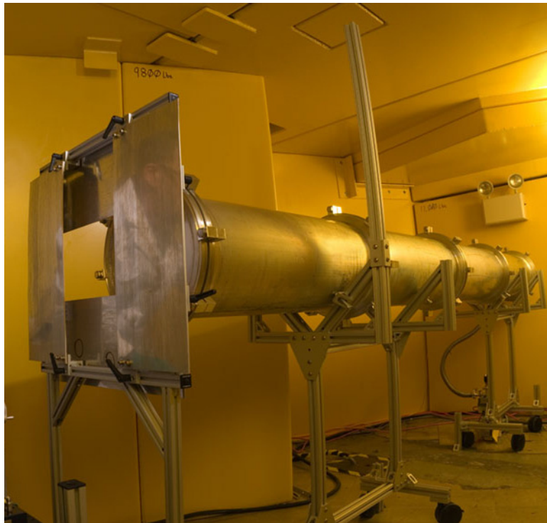
Figure 3.7. Flight tube for the Neutron Imaging beam line with adjustable beam aperture (Jacobson 2007).
