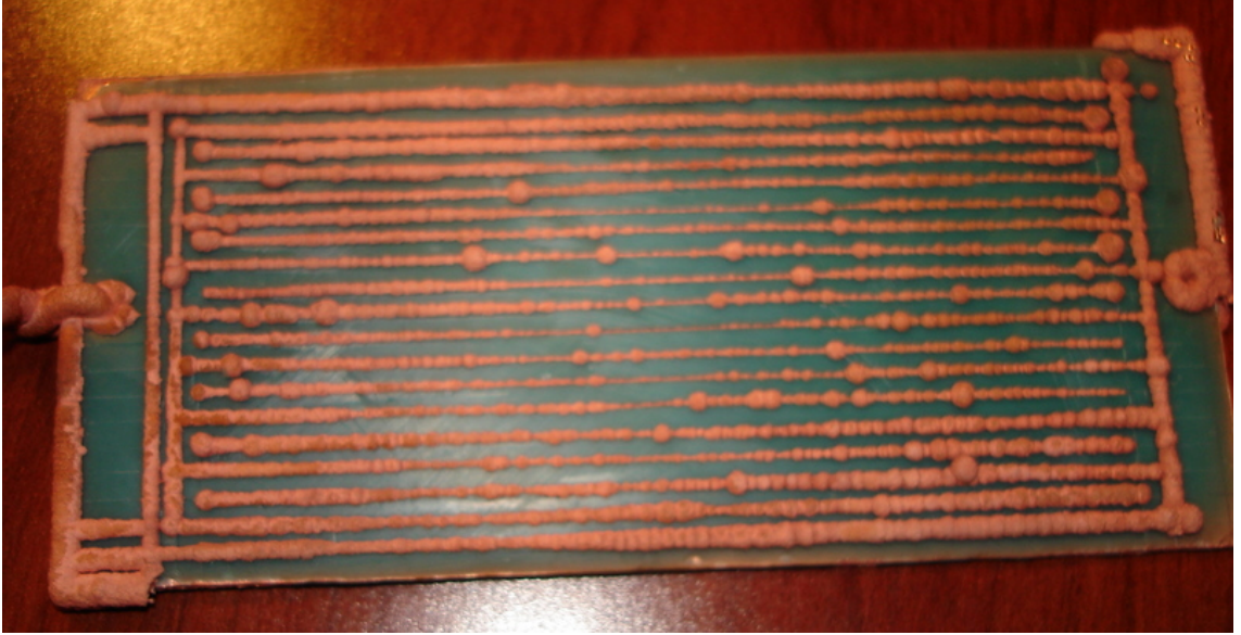
Figure 2.8.: TCV-2.0 after electroforming of the channel walls - notice the lumpy dendritic growth on the walls.
