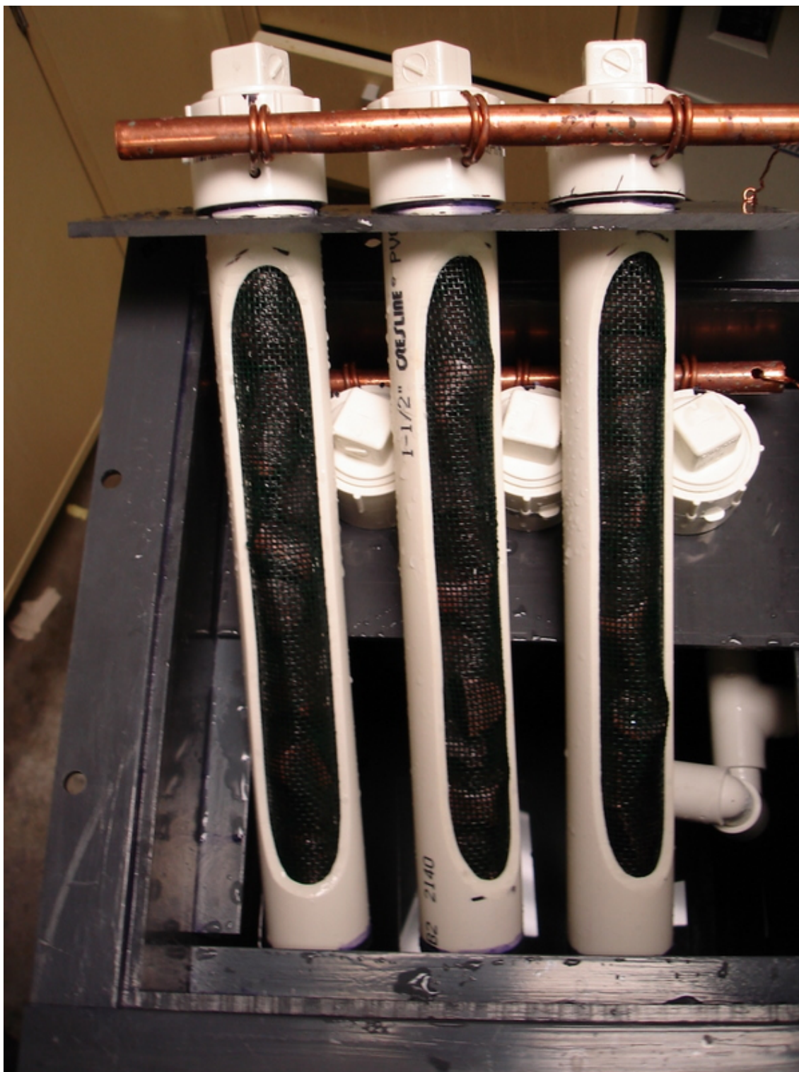
Figure 2.3.: Photo of one half of the anode bank, containing 3 anode tubes, with the electroforming bath in the background. (Anode bank consists of 1.5" PVC pipes with 1/3 removed from one side. Inside are phosphorized copper nuggets that are used as the sacrificial anode media. To maintain a conductive path there is a small copper tube inside the PVC tube that connects to the buss-rod. The buss rod connect one side of anode tubes and is connected to the positive side of the power supply.)
