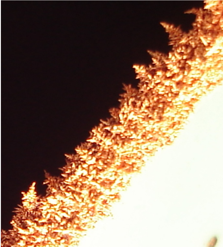
Figure 4.1.: Edge of plate TCV-2.1. The green color is the wax used to mask the back of the copper plate and prevent the plating from growing on the back side. The fuzzy copper is clearly a crystalline dendritic structure.
