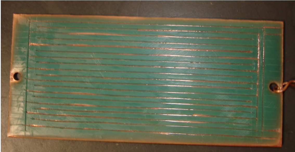
Figure 2.7.: Wall channels cut through the thick wax layer on copper substrate
