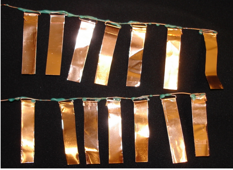
Figure 4.4.: Copper tabs attached to a copper wire for the purpose to testing the growth rate of the electroforming bath.
