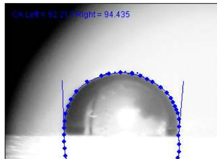
Sol-gel film with 5wt% organo-silicate particles
