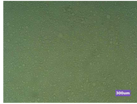
3% Teflon:PGMEA:PPG = 3:1.5:0.75 At 20X (Contrast is very bad when glass samples are used)
