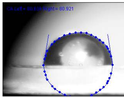
Sol-gel Ctrl #2 (0wt% particles loaded)
