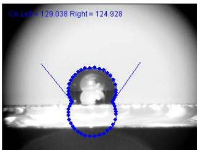
0.25%(wt%) SiC added, 4000RPM CA 125~129
