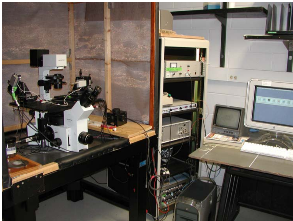
Fig. 1.2 A typical exocytosis measurement setup based on a patch-clamp system. From left to right is: Faraday cage shielded microscope bench with piezoelectric micromanipulator and head stage preamplifier; instrument rack of patch-clamp amplifier, AD/DA module, monitor etc.; computer control for voltage/current clamp and data acquisition. (Courtesy of Dr. Gillis's electrophysiology lab at Dalton Cardiovascular Research Center)
