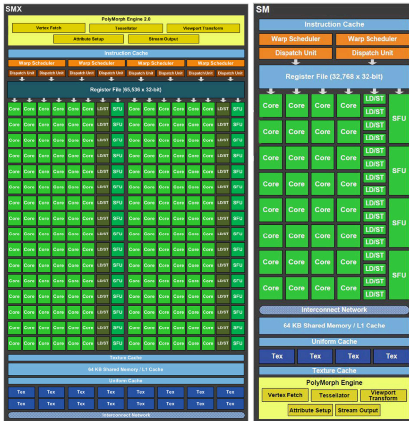
Figure 2: Kepler GPU architecture and SMX v.s. Fermi's SM
