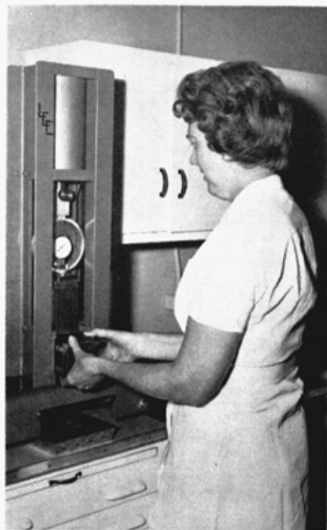
Above: Research home economist using a shear process to measure the tenderness of meat samples cut from roasts prepared by different cooking methods.
