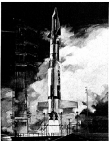
Dyna-Soar manned space glider is shown, in artist's concept, atop Titan ICBM for launching. Design will permit return for conventional landing. Boeing is prime contractor for glider and system.
