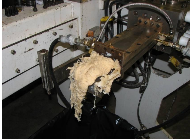
Figure 4.16 Extruded soy meat analog as it flows from the extruder barrel.
