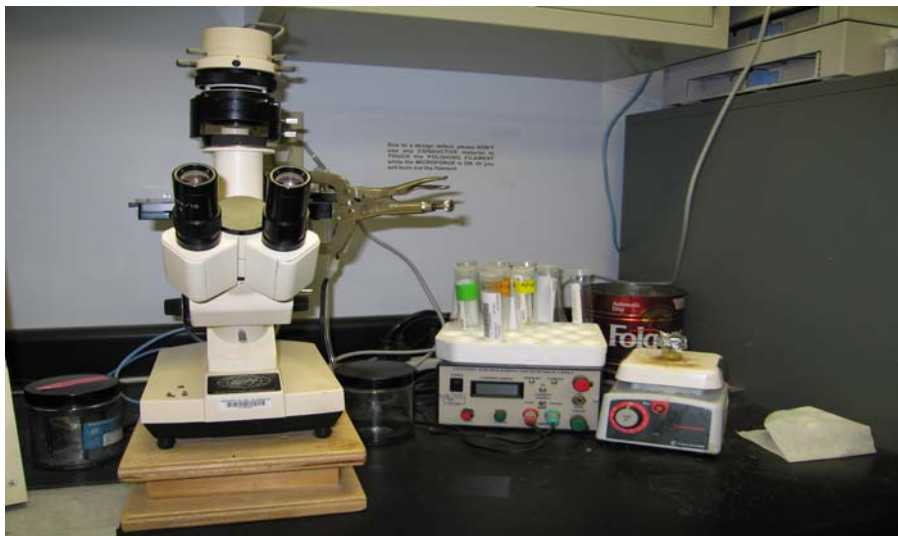
Figure 2.1. CPM-2 Microforge (Dr. Kevin Gillis lab, University of Missouri).
