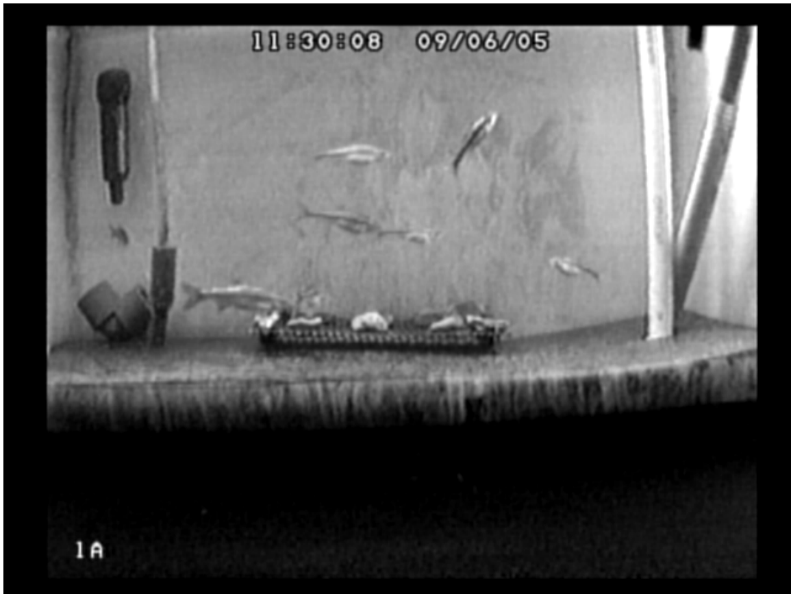
Figure 1: Still image of experimental tank design used in Experiment 1 (8 treatments; 4 temperatures and 2 photoperiods). Shown are the plexiglas false floor and the egg-collection dish in the rear-middle of the tank.
