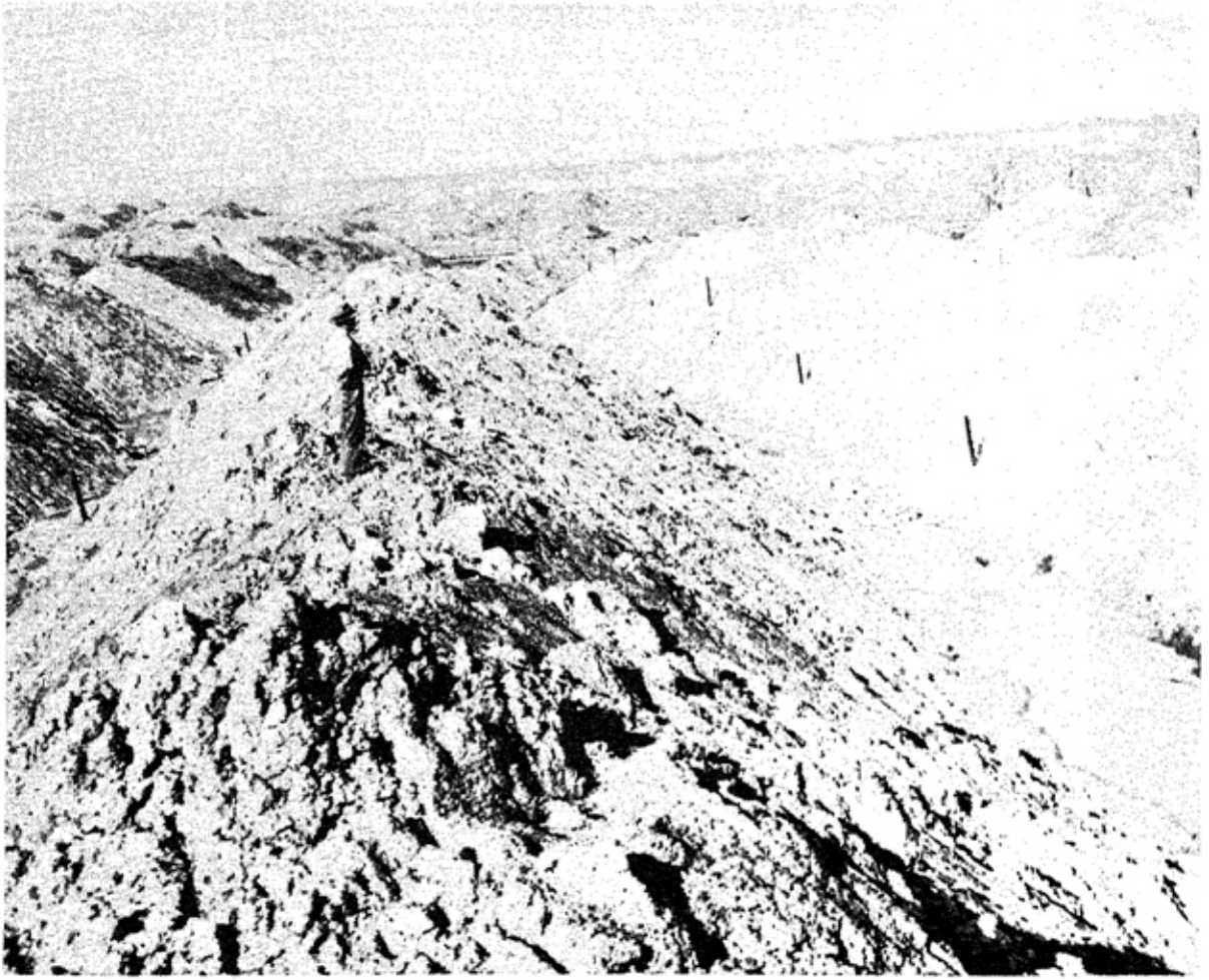
Figure 7.—Mine banks created by a dragline and a shovel working in tandem, Henry County, Missouri. These new banks, less than 1 year old, are composed of more than 50 per cent soil-sized particles (less than 2 mm. in diameter), and have less than the average amount of stone on the surfaces.
