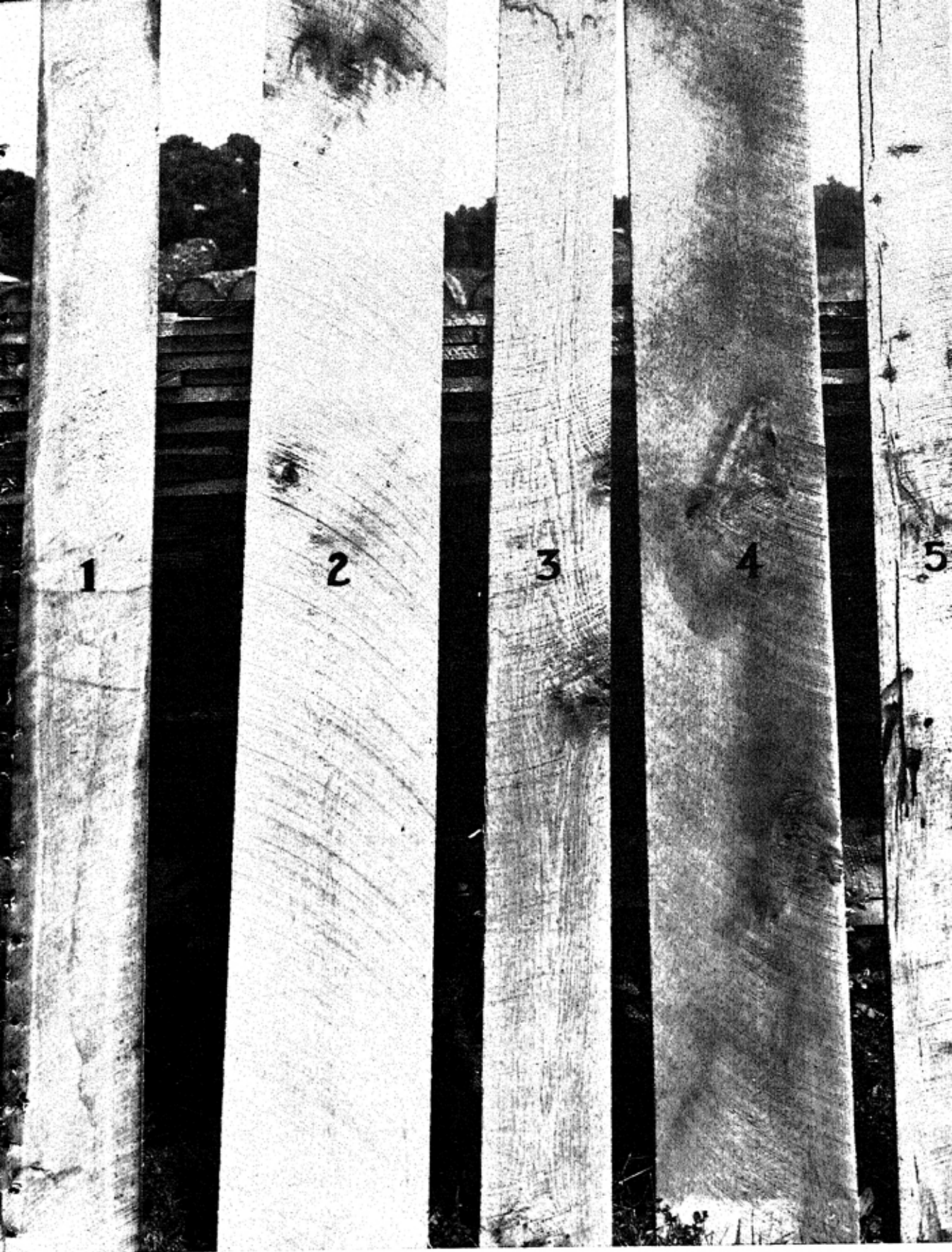
Figure 7—Five grades of lumber: (1) Second (2) No. 1 Common (3) No. 2 Common (4) No. 3 A Common (5) No. 3 B Common.
