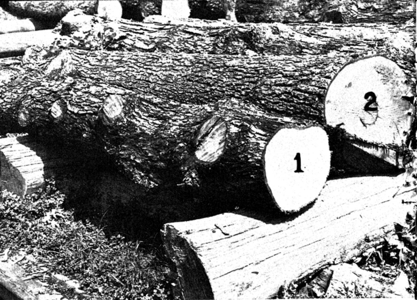
FIGURE 1 —Log 1 is a cull because knots are spaced less than 2 feet apart. Log 2 is a No. 2 log because it has one clear face. Its quality is lowered by a butt fire scar.
