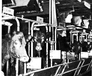
Figure 7—Interior of radiation chamber. From left: Control cows, F-235, F-282, and F-324, with dummy heat sinks suspended above them; experimental cows, F-246, F-308, and F-335, with refrigerated heat sinks suspended above them. The polished aluminum partition between experimental and control cows appears in center.
