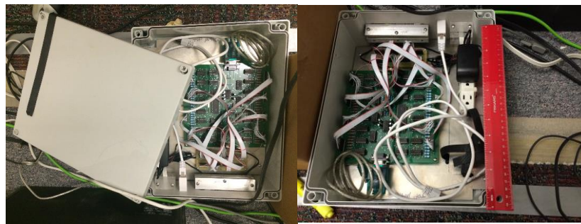
Figure 4-23 the Commercial electrical box for PSoC boards. Two processing boards can be put in a commercial electrical box.
