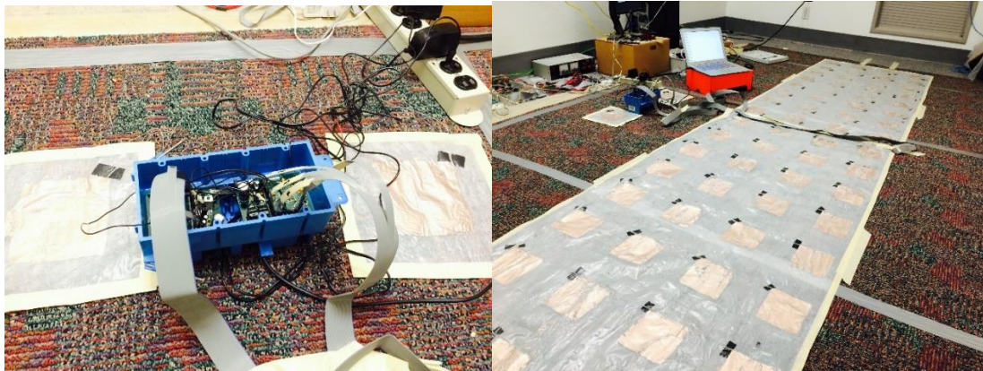
Figure 3-53 shows the 64-sensor signals scavenging system. The two individual 64 sensors are used as reference sensor for each board differential amplifier. The two boards are powered by a 5-volt power adapter. Each board is connected to one sensor segment shown on the right.
