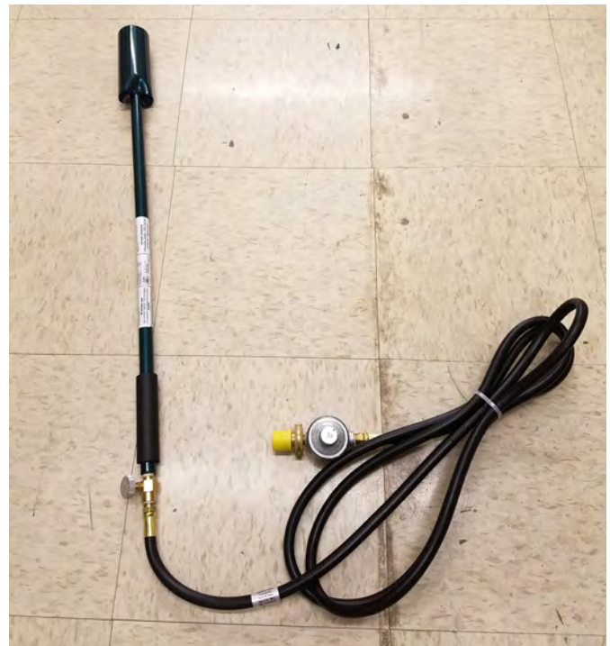
Figure 1. A basic torch apparatus consists of a hand-held wand attached to a hose, as pictured, that is connected to a standard 20-pound propane tank.
