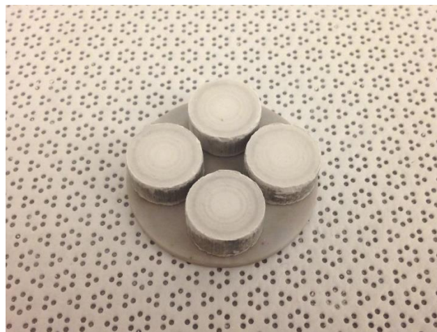
Figure 2.7 Ceramic green body prepared with corn starch
