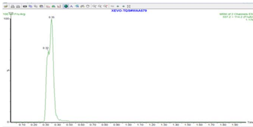
Figure 4.4 MRM chromatogram of FruArg using a water and acetonitrile gradient.
