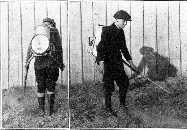
Fig. 15.—Bellows type dusters for applying dust mixtures on potatoes or other garden crops.
