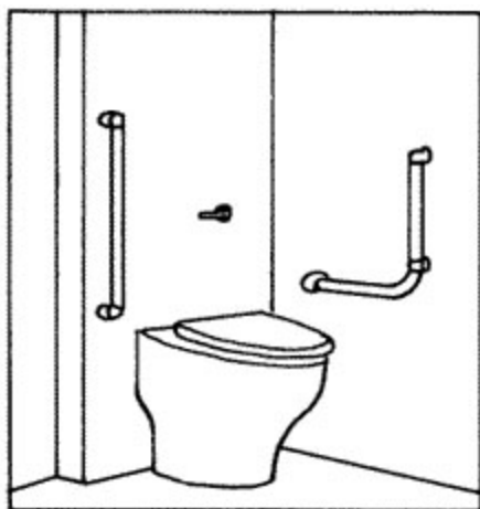
Figure 13 Side and back mounted bars.
