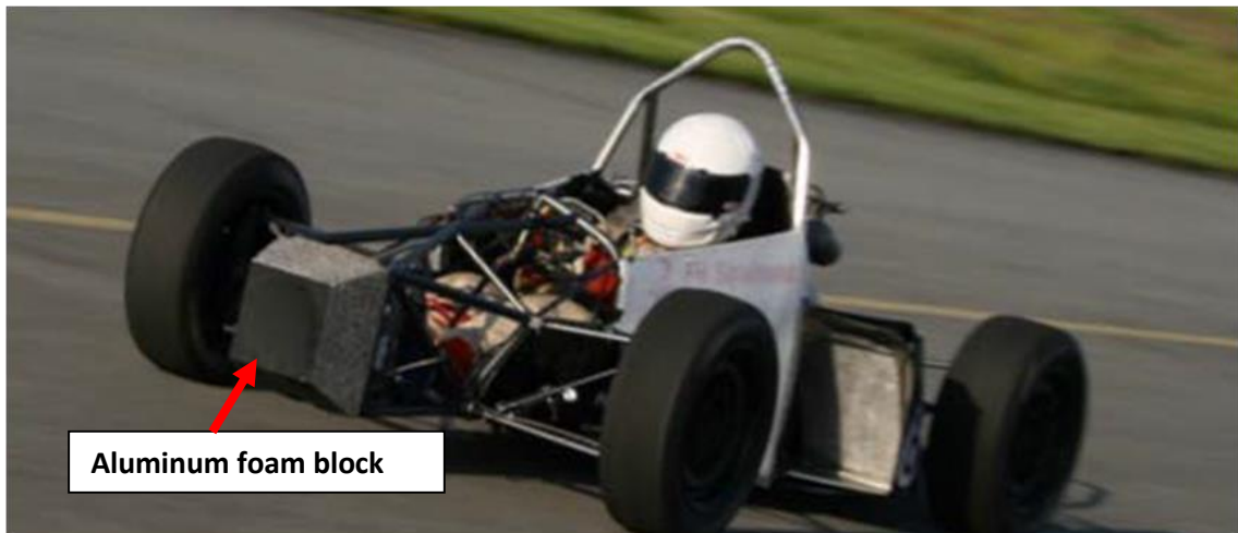
Fig. 2.14. Crash protector in a model racing car built by students at the University of Technology of Stralsund, Germany; a) view of car with the front encasement taken off. [80]
