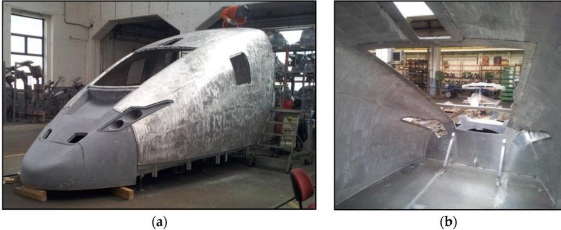
Figure 2.8. (a) Prototype of German high velocity train ICE made of welded aluminum foam sandwich; and (b) view of the interior with the low number of components required (courtesy of Thomas Hipke, IWU, Chemnitz, Germany and Voith Engineering, Chemnitz, Germany). (79)
