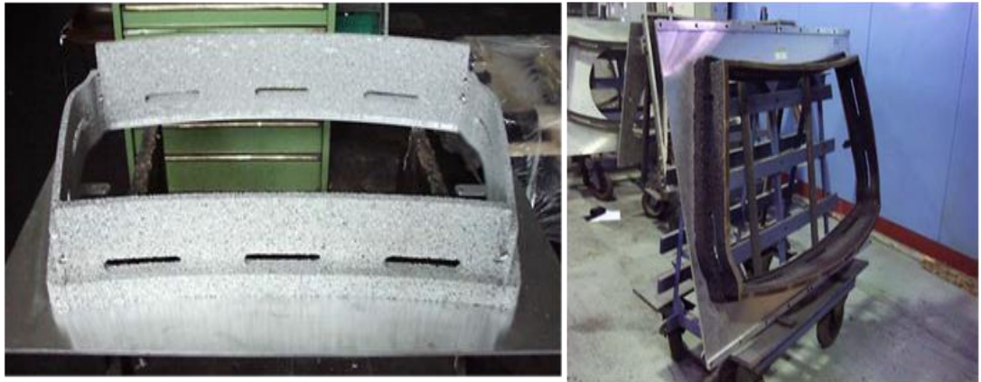
Fig 2.12. Vacuum lifting tool for Pilkington containing an Alporas aluminum foam ring (79)
