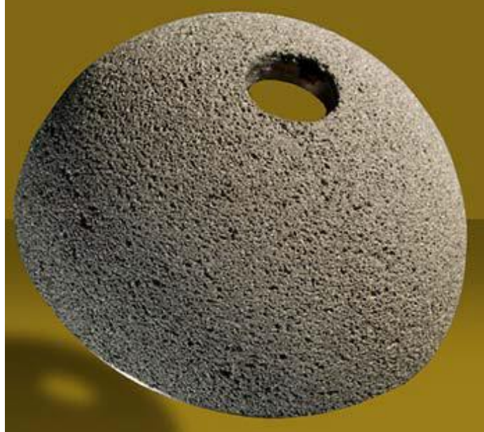
Fig. 2.15. Porous titanium coating on an acetabular cup for hip replacement (Courtesy of National Research Council Canada, Industrial Materials Institute) (80)
