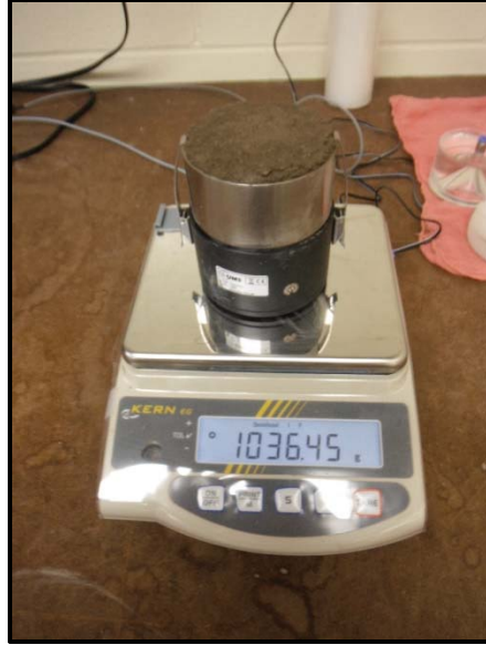
Figure 3.18: "HYPROP" Test Specimen and Evaporation - Measurement Process in Progress
