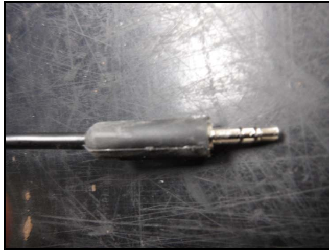
Figure 3.6: Stereo Plug Connecting Sensors to Decagon Devices "EM50" Data logger
