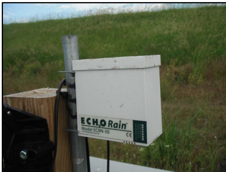
Figure 3.10: Decagon Devices (Decagon, 2012) "ECRN-50 Low-Resolution Rain Gauge" Sensor Used to Measure Precipitation
