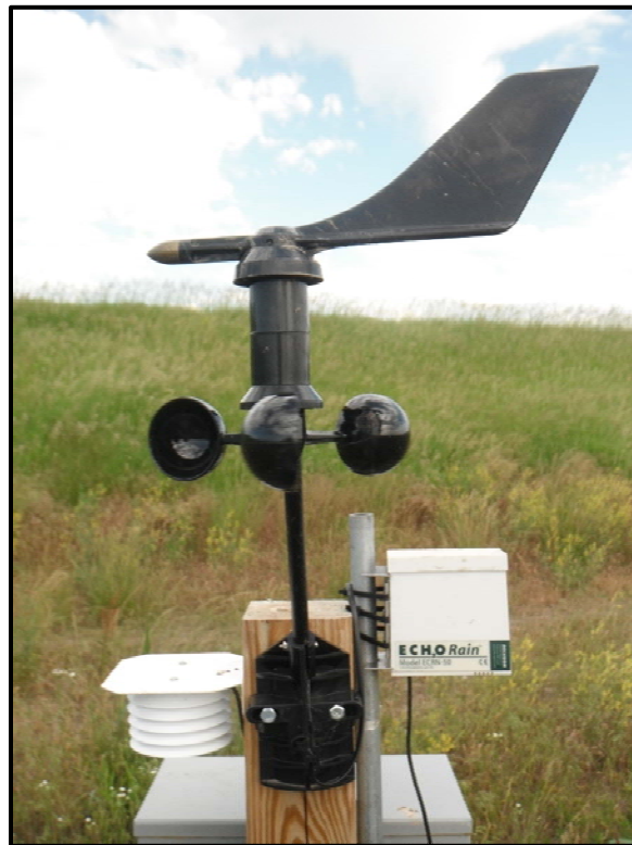
Figure 3.11: Decagon Devices (Decagon, 2012) Davis Cup Anemometer Used to Measure Wind Speed and Direction
