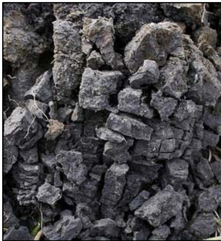
Figure 5.19: Blocky Soil Structure from Test Pit No. 2 of McBaine, MO Soil at a depth of 6 in.
