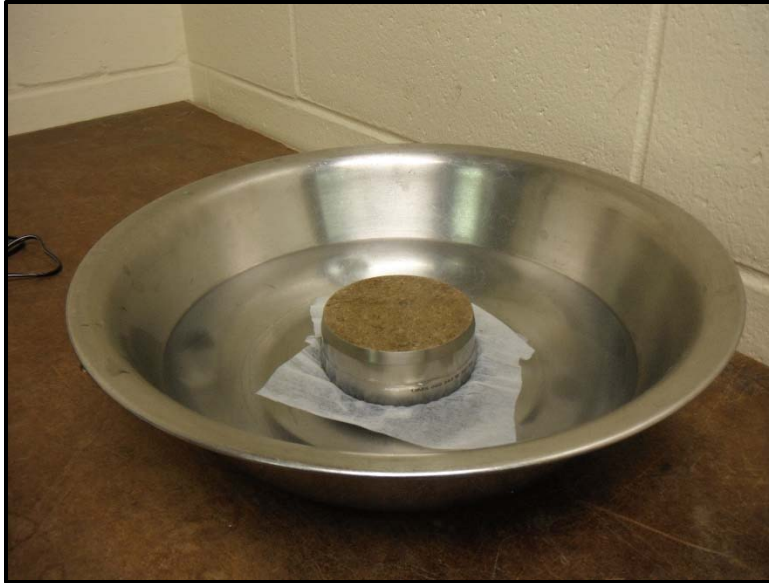
Figure 3.16: Soil Specimen Saturating in "HYPROP" Sampling Ring
