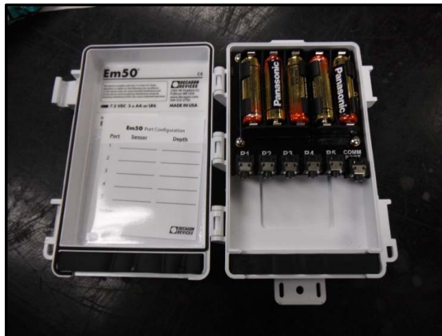
Figure 3.7: Decagon Devices "EM50" Data logger Used to Store Sensor Measurements
