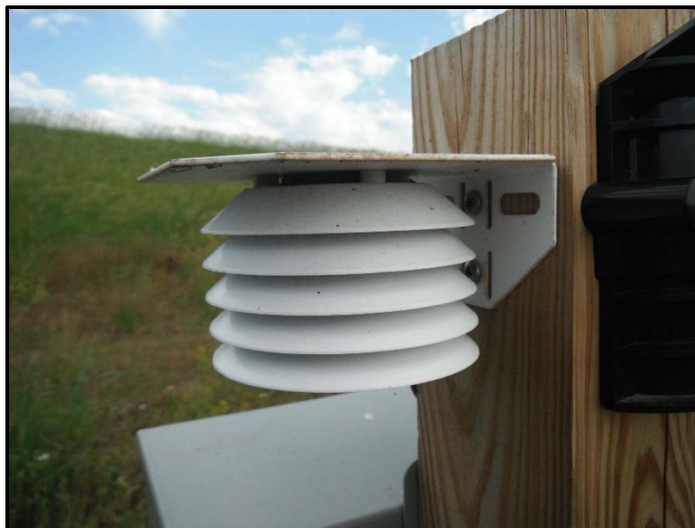
Figure 3.13: Decagon Devices "VP-3" Sensor Used to Measure Air Temperature and Relative Humidity
