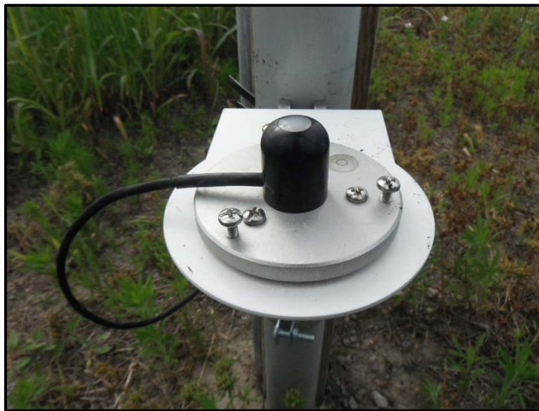
Figure 3.12: Decagon Devices "PYR Total Solar Radiation" Sensor Used to Measure Solar Irradiance
