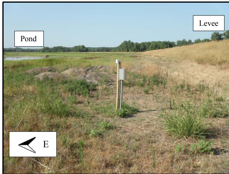
Figure 3.3: Instrumentation of Test Site 25 ft. off East Toe of Missouri River Levee System
