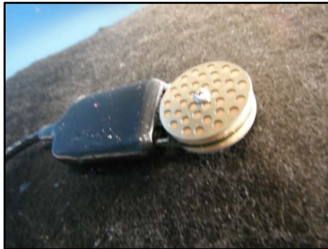
Figure 3.9: Decagon Devices "MPS-2" Sensor Used to Measure Matric Suction and Soil Temperature
