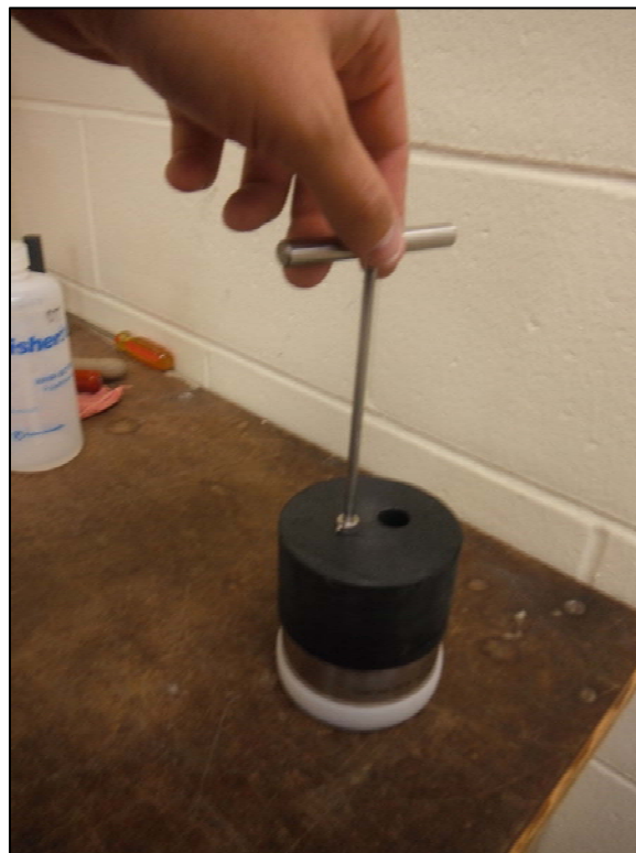
Figure 3.17: Drilling Pilot Holes in "HYPROP" Soil Specimen
