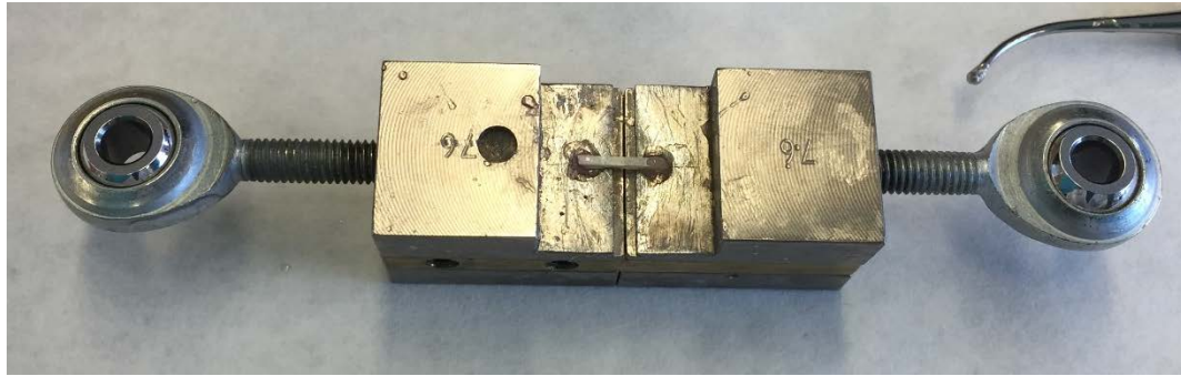
Figure 2. Example of Beam Attached to Microtensile Tester Fixture.
