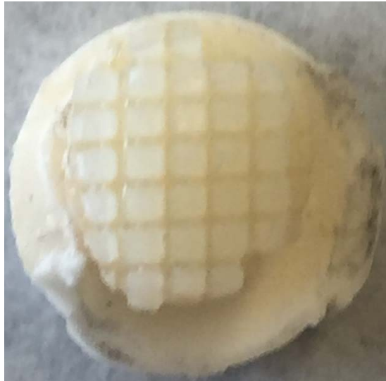
Figure 1. Example of Specimen Preparation. Beams before removing from tooth root.
