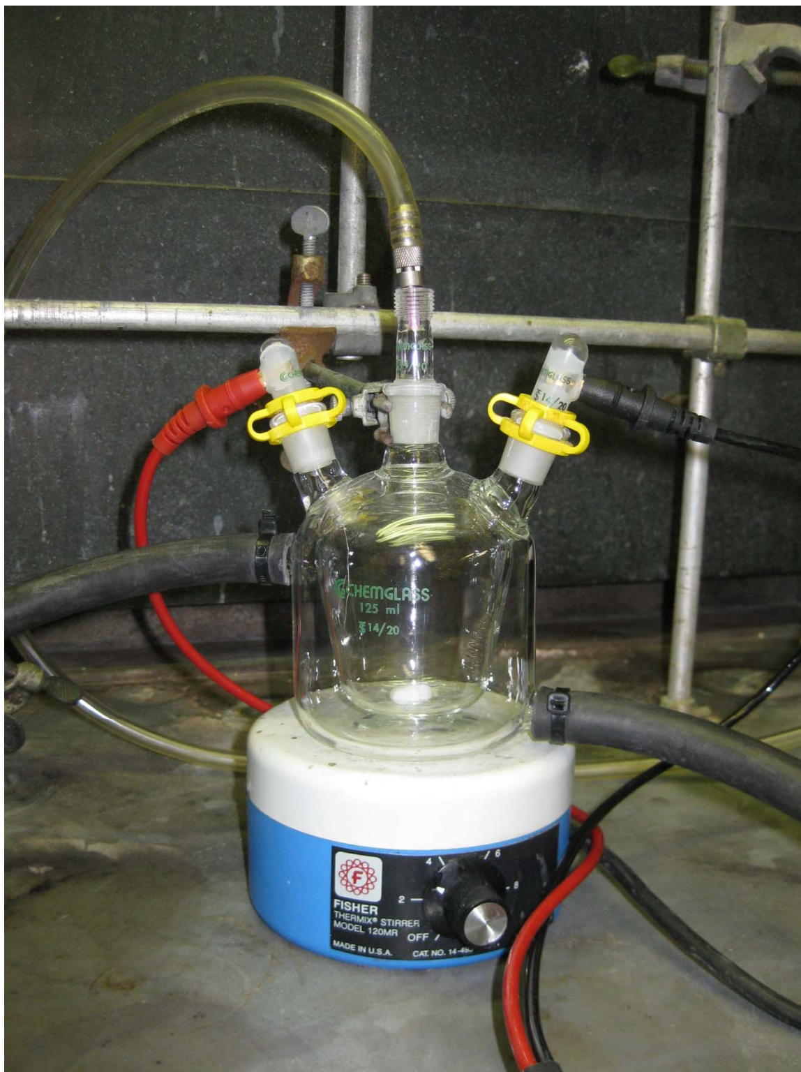
Figure 2.6 Close-up of jacketed electrolysis vessel for preparation of peroxymonophosphate.
