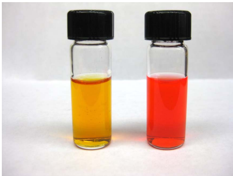
Figure 4.3 Color change resulting from treatment of PC-1 with hydrogen peroxide. Left: 1 mM solution of PC-1 in 50 mM Bis-Tris pH 7.0. Right: 1 mM solution of PC-1 in 50 mM Bis-Tris pH 7.0 treated with 10 mM H 2 O 2 for 1h.
