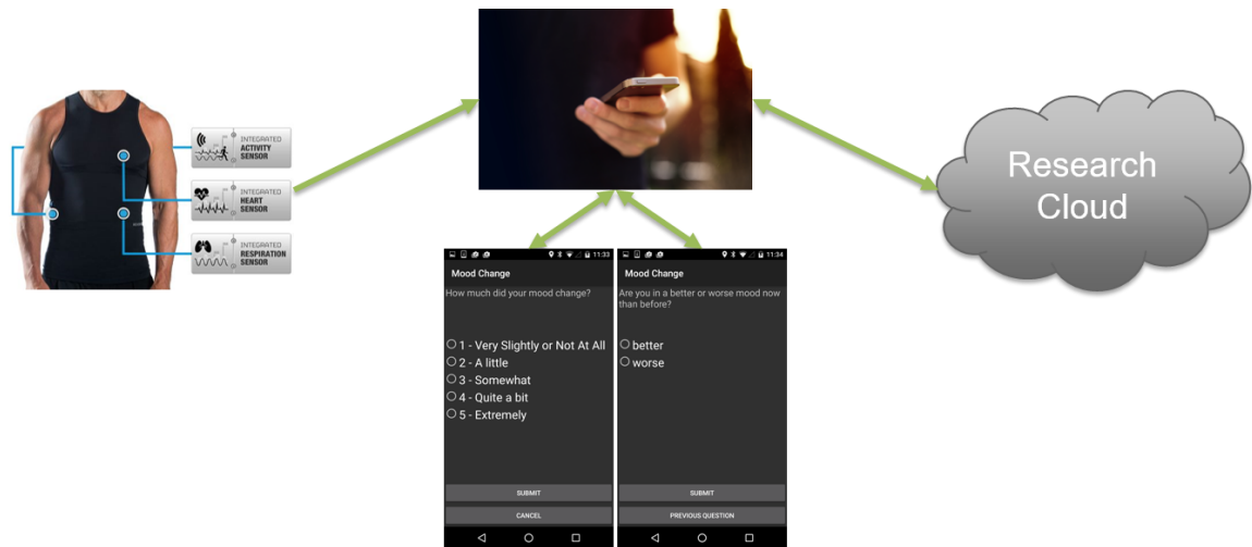
Figure 19. A flow chart of the mobile ambulatory assessment system (mAAS) and the three main components: External sensors, mobile devices, and cloud web servers. The surveys managed by the smartphone are used to determine the emotional state of the subject used in the Analysis of Mood Dysregulation (AMD's) pipeline.
