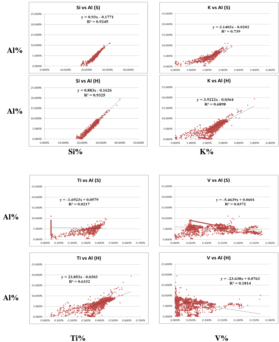
Figure 4.6. Correlation between Al and other elements (Si, K, Ti, V, Ni, Co, Cu, P, Zn, Pb, Sc, La and Sb) in Hushpuckney (H) and Stark (S) black shales. Strong Al-Si correlation is expected if clay minerals are present. A strong positive Al-K correlation is expected if illite is present.
