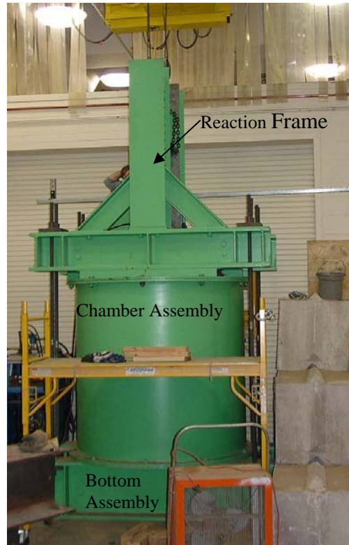
Figure 3.1. Photograph of the experimental setup showing the bottom assembly, chamber assembly, and Reaction Frame.
