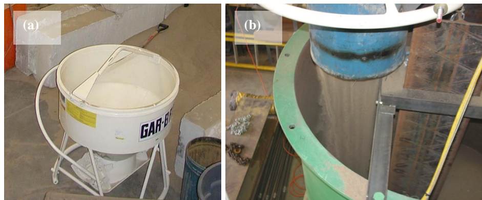
Figure 3.16. Photographs of (a) the dump bucket, and (b) soil being placed into the chamber using the dump bucket and sieve.
