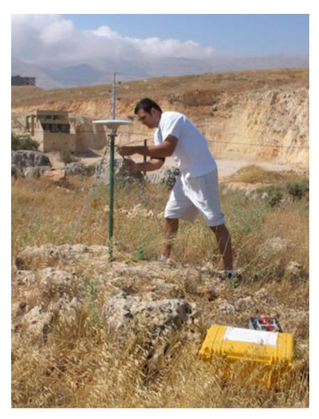
Figure 3.1: Fixed height mast with Zephyr antennae installed at HZRT.
