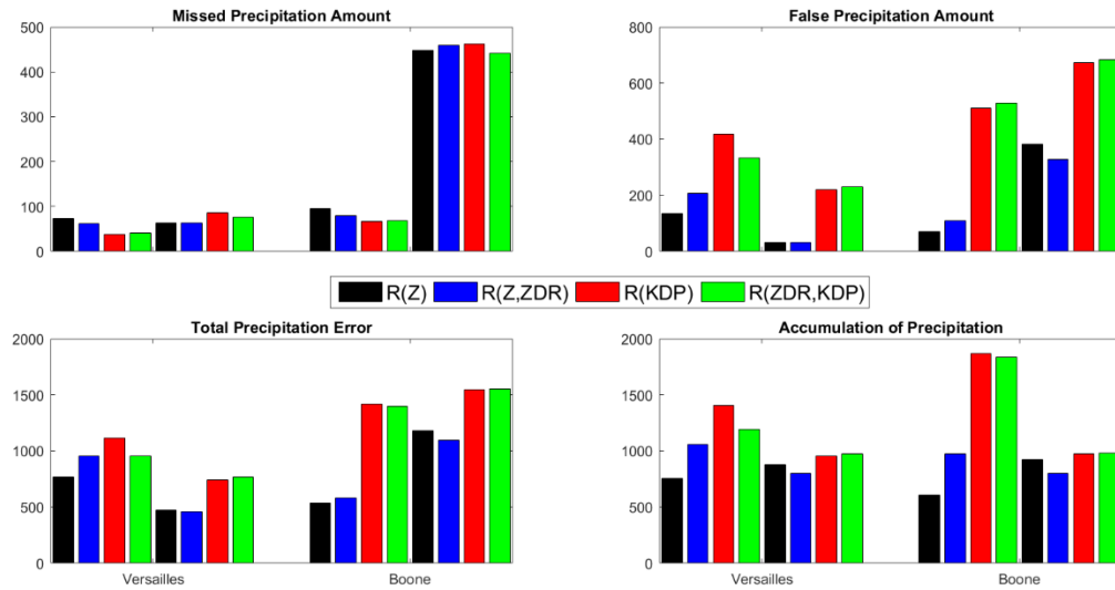
Figure 3B.11. Quantitative analyses between the MZZU X-band and Kansas City (KEAX) S-band radars. Distances from the Versailles and Boone sites were 72 and 130, and 5 and 173 km for MZZU and KEAX, respectively. The four results to the left and right of each location represent results from, respectively, MZZU and KEAX.
