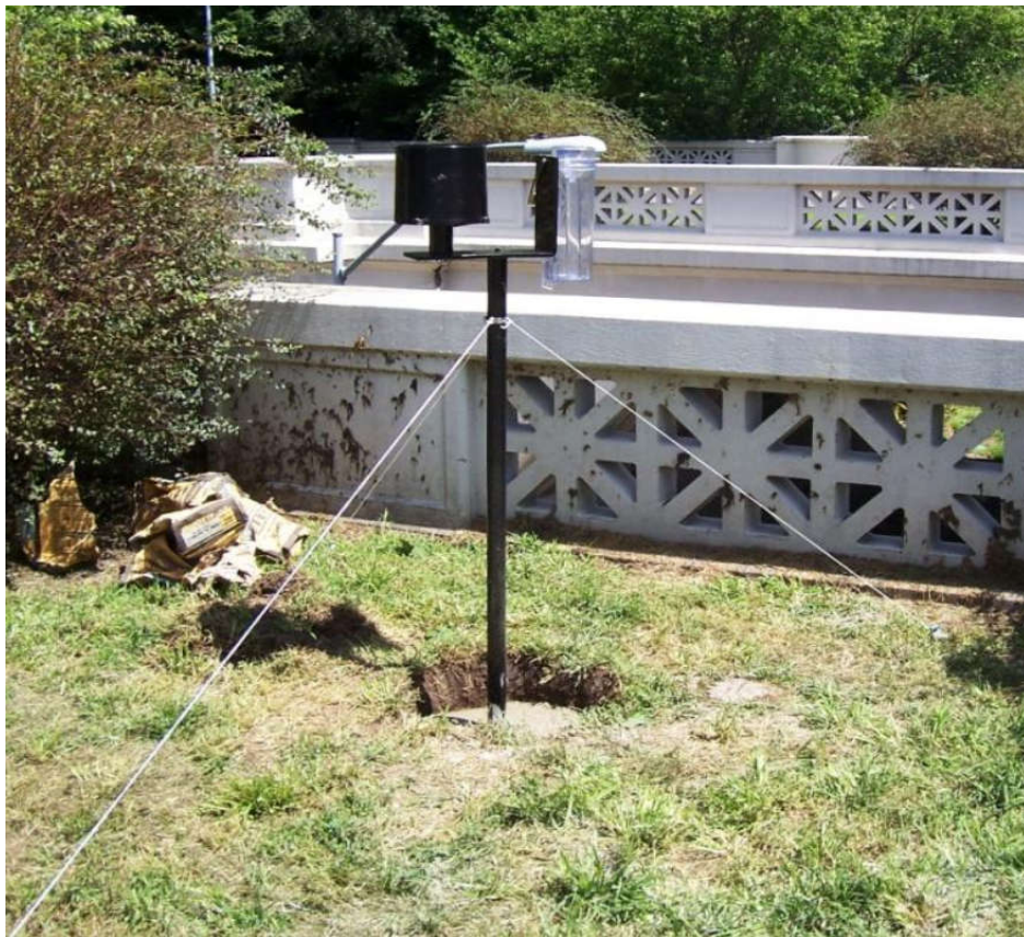
Figure 2.4: Rain Gage Installed at 77 th and Paseo (Source: Ma)
