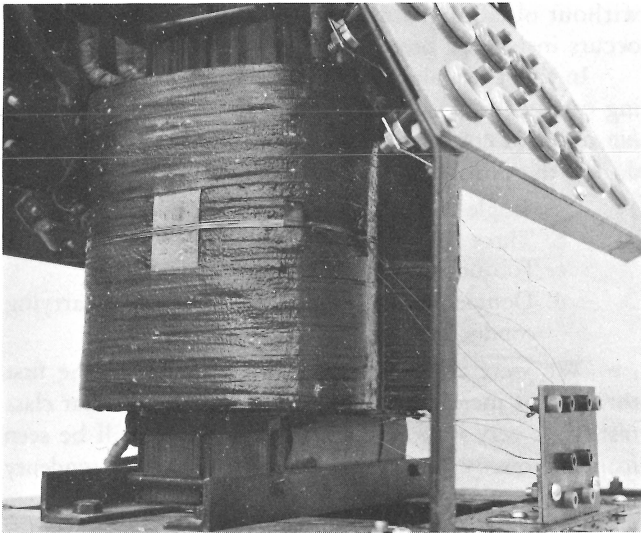
Fig. 1. Single phase core type commercial transformer with search coils added to demonstrate leakage flux.
