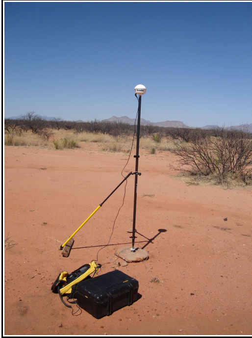
Figures 3.1A and B. A) The base station is a Trimble ProXRS backpack L1 capable unit. B) The rover is a Trimble Ranger with Hurricane antenna, also L1 capable. Each unit is pictured set up at an ASA point on the East Range of Fort Huachuca.
