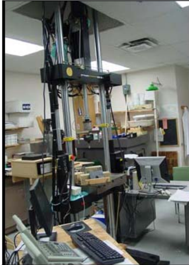
Figure 4. Instron 8821s servo-hydraulic testing machine in the biomechanics lab of the Comparative Orthopaedic Laboratory (COL). For this project, the machine was equipped with a 1000 N load cell attached to the ram which has a maximum ram travel of 260 mm. A stainless steel impactor (tip diameter of 3.9 mm) attached to the end of the ram (below the load cell) and a stainless steel base (containing a stainless steel anvil with specimen-restraining well located in the center) was attached to the test table (See Appendix B for detailed fixture drawings).
