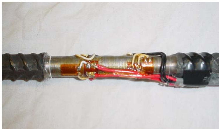
Figure 3.2 – Instrumented Rebar showing installed strain gages
