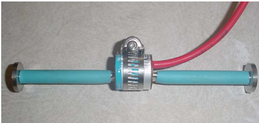
Figure 3.3 – Model 4200 vibrating wire gage from Geokon Incorporated
