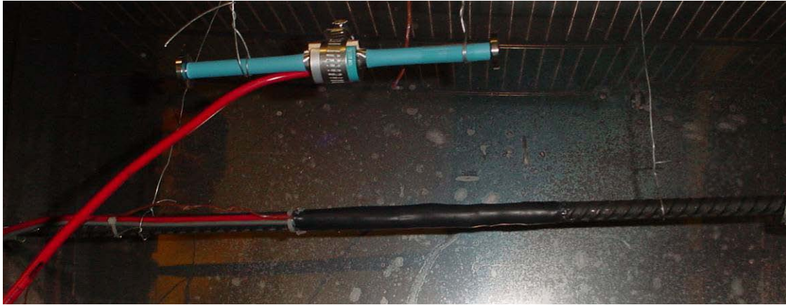
Figure 3.11 – Unrestrained instrumented rebar and vibrating wire gage in temperature controlled oven
