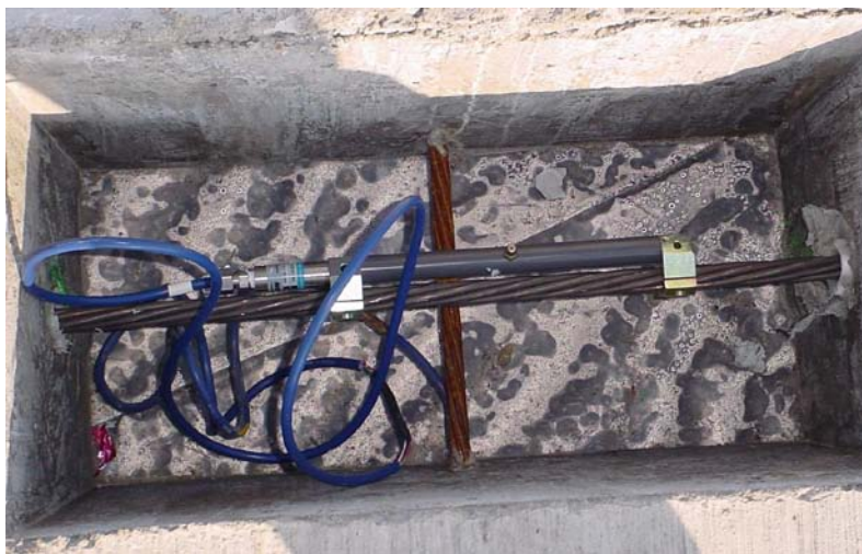
Figure 3.4 – Model 4410 vibrating wire Strandmeter, unsheathed
