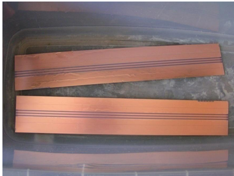
Figure 3-6. Exposed boards in the chemical bath.
