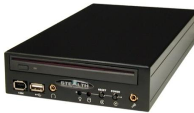
Figure 5-12. Photograph of Stealth computer used for data acquisition from temperature sensors.
