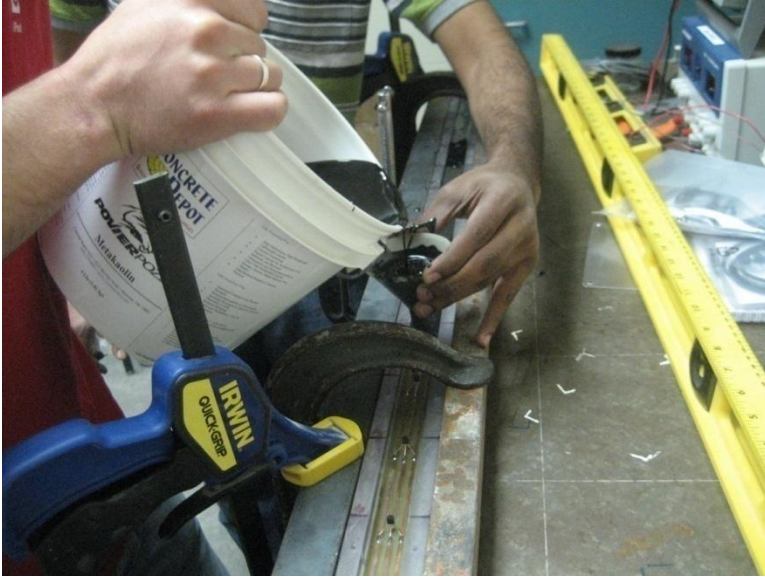
Figure 3-12. Pouring epoxy into large test array.
