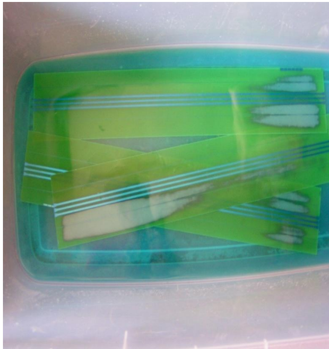
Figure 3-7. Excess copper being removed from the printed circuit boards.
